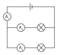
The two lamps in this circuit are identical.
