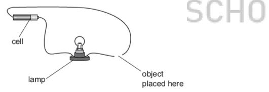
Oliver places different objects between the wires.
